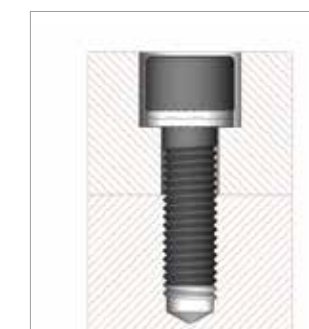
Countersunk socket head bolt secured in position
