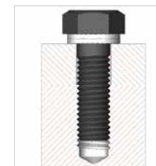
Hexagon bolt secured in a blind hole
